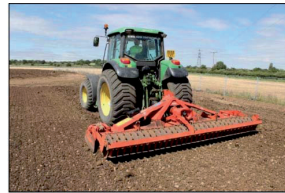
Figure 25 power-harrow being used to cultivate topsoil on the Stadium Pitch.
